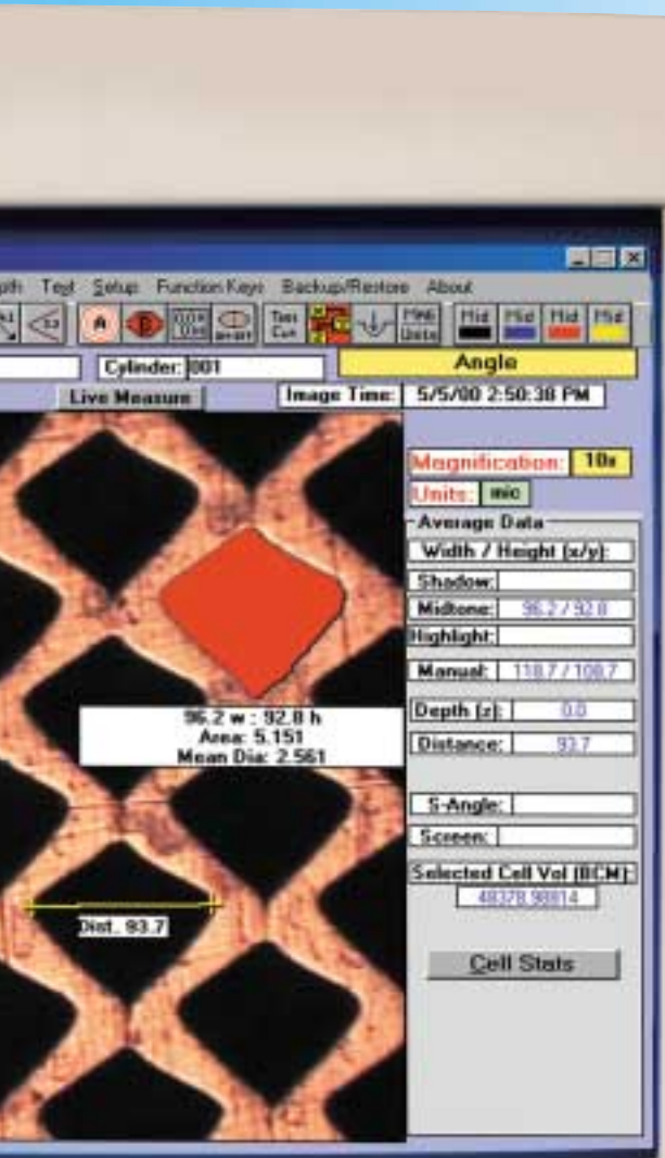
▲ Laser engraved cells on anilox roll
